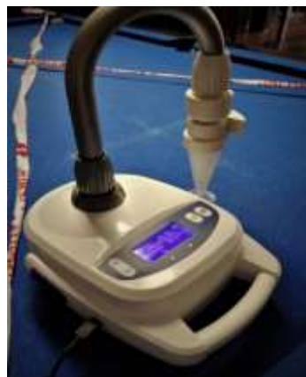
Figure 5.3- Liquid Impinger Coriolis with NVL inactivation buffer (Nzytech genes & enzymes) during a FFH SARS-CoV-2 sampling campaign.
