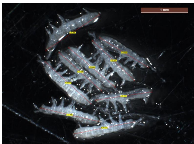
Figure 2.4 - Measurement of body size on Folsomia quadrioculata , using Leica Application Suite software. Author's original.
