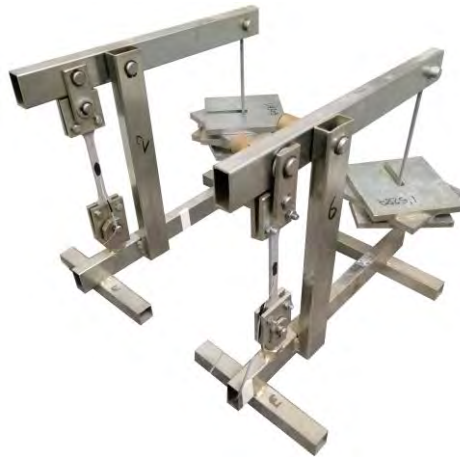
Figure 3.11. Time-dependent tension test setup for epoxy specimens.
