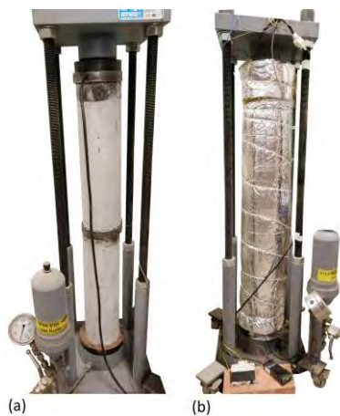
Figure 3.4. Creep specimens at: (a) 20 °C and (b) 50°C.
