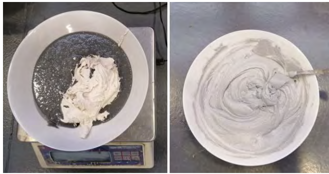
Figure 5.1. Epoxy adhesive mixture.
