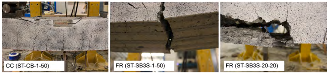
Fig. 8. Representative views of failure modes of specimens in Series 1.
