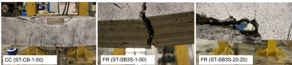
Figure 6.8. Representative views of failure modes of specimens in Series 1.
