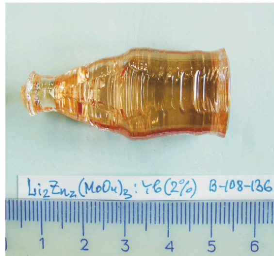
Figure 1. Photograph of the as-grown boule of the \text{LiZnMo} crystal doped with (nominally) 2 at.% \text{Yb} ; the growth direction is along the [010] axis.
