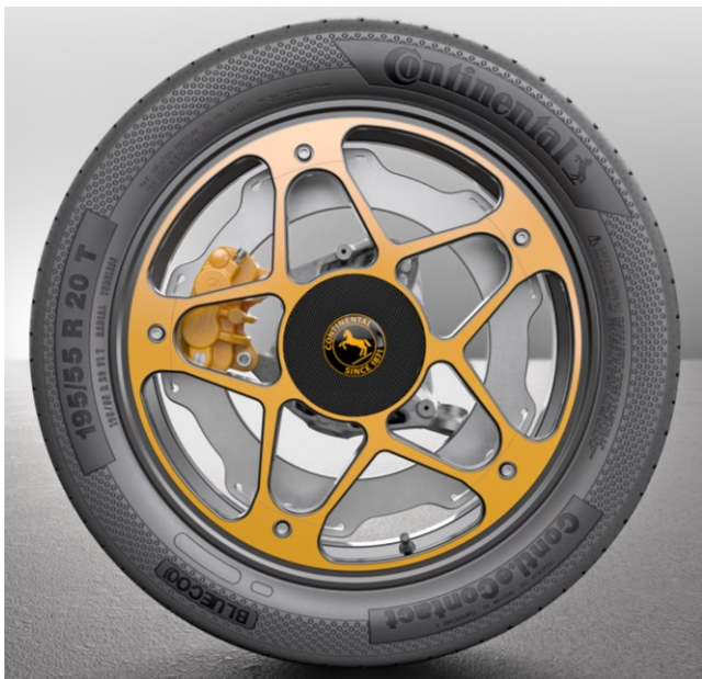
Figure 2-7: New wheel concept with aluminum brake disc and an inside out floating caliper 31
