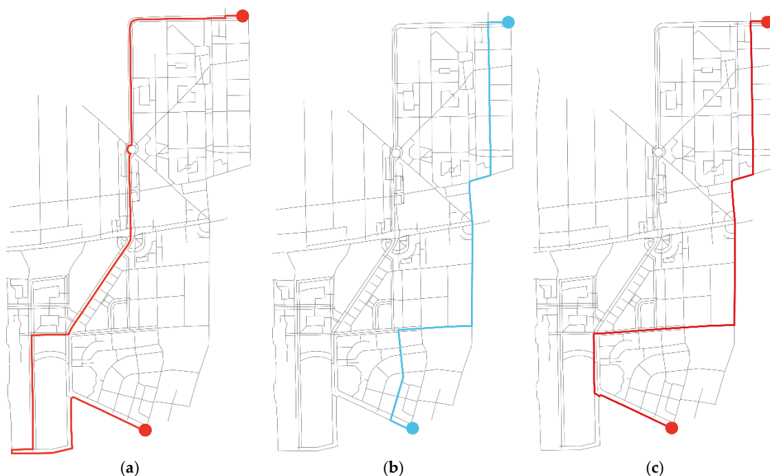
Figure 3. Shortest path findings with the influence of (a) the shortest block-distance path from two points; (b) choice in between; (c) the fewest number of turns path from two points.
