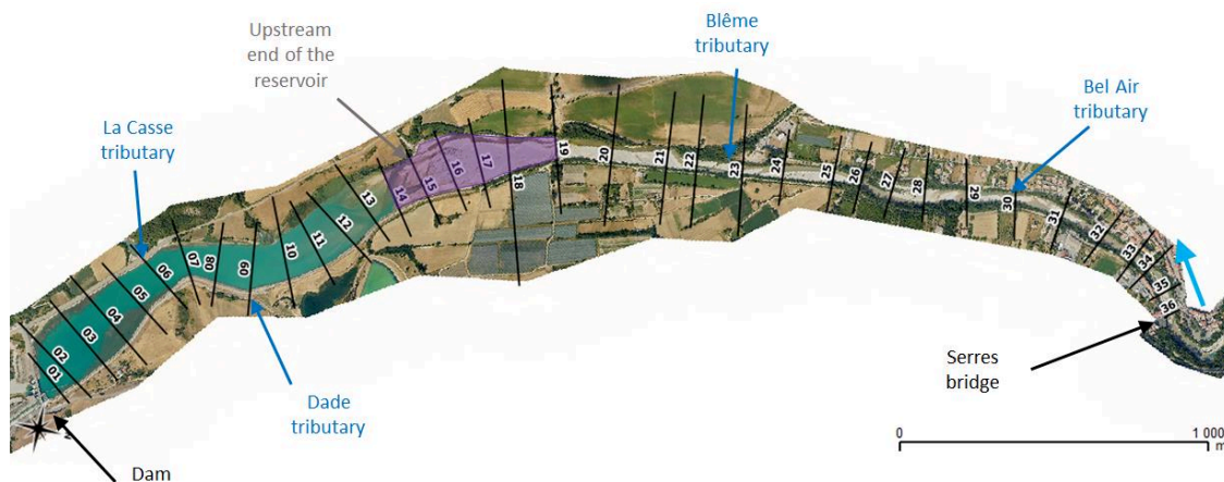
Figure 2. Presentation of the study site. The black lines indicate the cross-section locations of the bathymetric surveys. The purple polygon corresponds to the dredged area at the upstream end of the reservoir.
