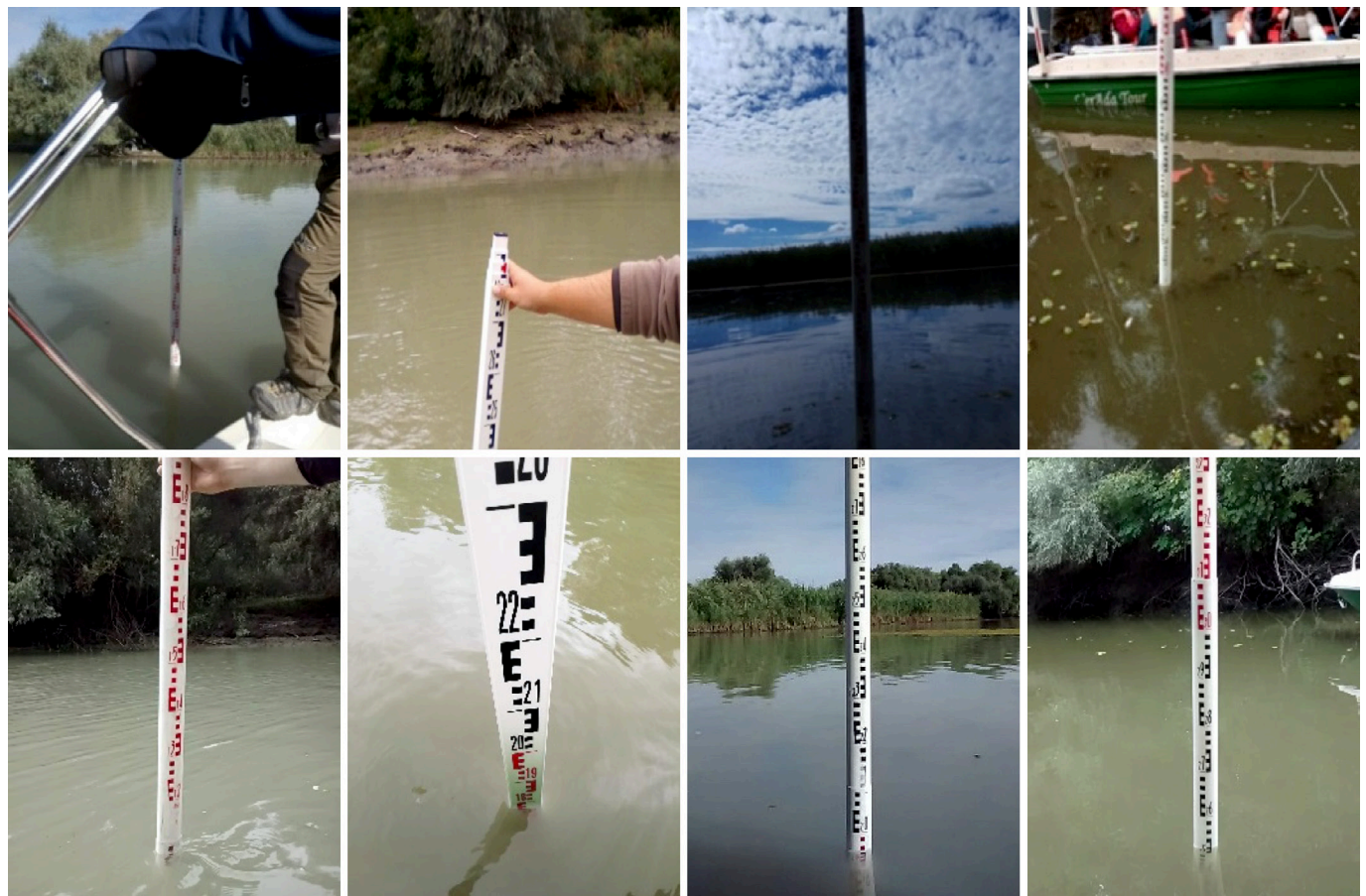
Figure 4 | Collected water levels of bad quality (upper row) and good quality (lower row).
