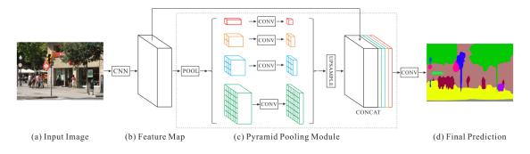
Figure 4.2: Overview of the PSPNet architecture. Reprinted from [89]
