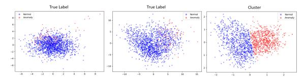
Figure 5.8: The left image shows the latent space of a VAE with a latent feature map of size 64 \* 4 \* 4. This latent space is significantly less suited to detect anomalies by clustering compared to the one in the middle which is produced by a VAE where the latent space has the size 512 \* 4 \* 4. The image on the right shows the latent space from the middle after clustering.
