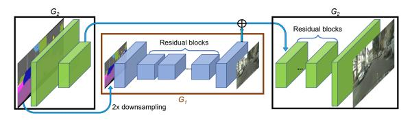
Figure 4.3: Pix2PixHD architecture. The residual network G1 gets trained on images with lower resolution. Later, another residual network gets appended and the networks are trained together while the input of the second part of G2 is the sum of the last feature map from G1 and the feature map from G2. Reprinted from [82]
