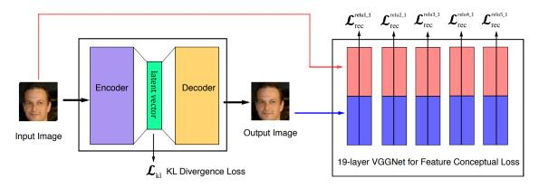
Figure 4.7: Overview of the feature loss. The feature loss gets calculated after every layer of the CNN (VGGNet) by taking the squared distance between the feature maps generated from the input and the reconstructed image. Reprinted from [43]
