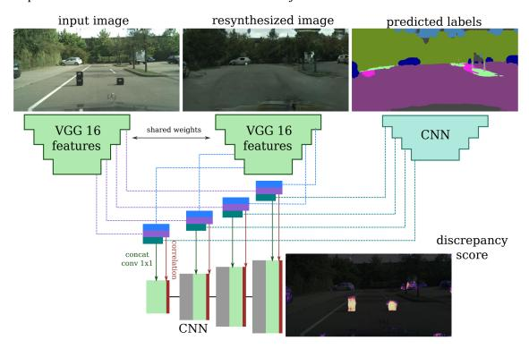
Figure 4.4: Architecture of the discrepancy module [51]. The VGG and CNN extract features from the three input images. Features and correlations are passed to a decoder which generates the final discrepancy map. Reprinted from [51]
