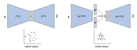
Figure 2.1: Basic architecture of AE/ VAE. On the left is a VAE where the encoder  $p_{\theta}$  calculates the parameters of a distribution from which the latent variable *z* gets sampled. The decoder  $q_{\phi}$  then tries to reconstruct the input *x*. On the right is a AE where the encoder produces *z* directly. As shown below, the latent space of a VAE is typically more meaningful and better structured when compared to an AE.
