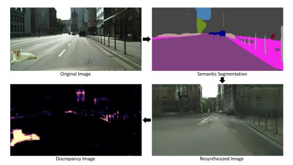
Figure 4.1: Overview of the pipeline which creates the discrepancy maps. The original image gets passed through a semantic segmentation module to create a semantic mask. From this a GAN tries to reconstruct the original image. The discrepancy map gets generated by comparing the original image to the reconstructed one.
