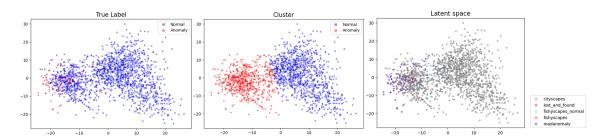
Figure 5.9: Latent space of a VAE with  $\beta$  of 0.01. The left image shows the true labels of the data and the middle one the cluster assignments. The image on the right shows to which dataset the individual points belong
