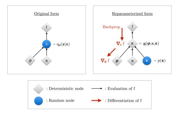
Figure 2.2: Illustration of the reparameterization trick. In the original form, calculating gradients for backpropagation is not possible because of the random variable *z*. In the reparameterized form, randomness is introduced with the help of an external node which makes backpropagation through *z* possible. Reprinted from [47].
