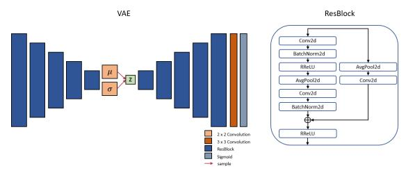
Figure 4.6: The left image shows the overall architecture of the VAE used in this thesis. The image on the right shows the components of the ResBlock.
