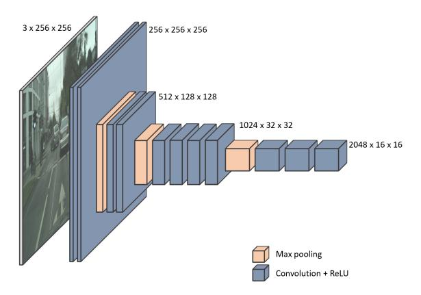
Figure 4.8: Architecture of the VGGNet to calculate the feature loss of a 256 x 256 rgb-image. The weights were taken from a network which was pre-trained on ImageNet and the the feature loss gets calculated after every convolution + ReLU block
