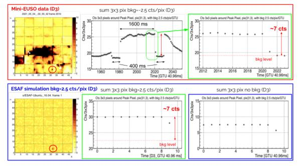
**Figure 6:** Top: Mini-EUSO flasher campaign event. Center shows the light evolution of summed counts of 3 by 3 pixels around the peak count pixel, indicated by red-circle on the left plot for a cycle of 1600 ms pulse. Transit of the 1600 ms pulse with 400 ms off before and after the pulse is clearly seen. Right shows the zoomed plot to the duration and timing where ESAF simulated the same event as shown in the bottom plots as following.
