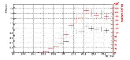
**Figure 2:** The detection exposure efficiency (on the left axis, in black) and geometrical aperture (on the right axis, in red) are shown as a function of the EAS energy logarithm. A UV background level of 1 photon/pixel/GTU was considered in both cases.
