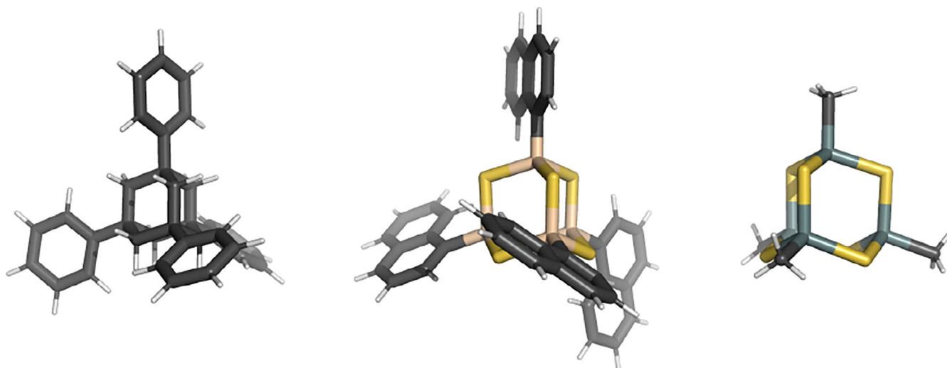
FIGURE 1 Minimum structures of cluster monomers optimized at B3LYP-D3(BJ)/cc-pVDZ(-PP) level of theory. Left: AdPh 4 , middle: [(NpSi) 4 S 6 ], right: [(MeSn) 4 S 6 ]. Color code: gray: carbon, white: hydrogen, yellow: sulfur, brown: silicon, blue: tin
