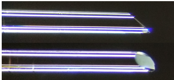
Figure 6. Angle polished PM fiber.
