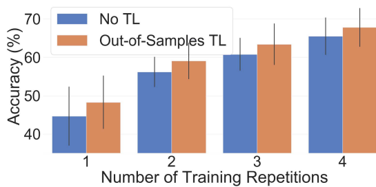
Fig. 5. Classification accuracy of the CWT-based ConvNets on the NinaPro DB5 with respect to the number of repetitions employed during training. The pre-training was done using the pre-training dataset . Training and testing only considered the 11 gestures from the NinaPro DB5 not included in the pre-training. The error bars correspond to the STD across all ten participants.
