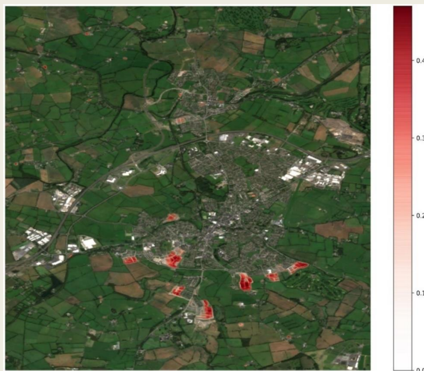
Figure 18. Urban expansion (2018-21) tracked in a settlement within the Dublin metropolitan area, based on probability-differences in the model's assignment of land use types to satellite image pixels.
