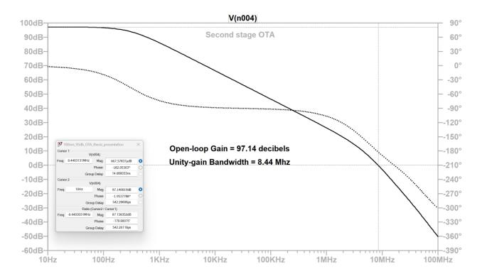
Figure 5.9: Bode plot for gain and phase of second stage
