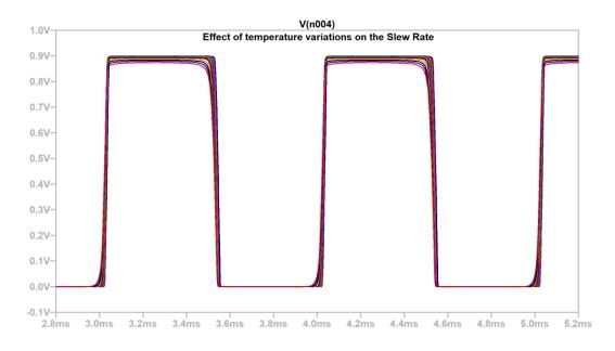
Figure 5.15: Effect of variation in temperature on slew rate
