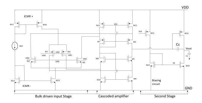
Figure 3.10 2-stage bulk driven OTA
