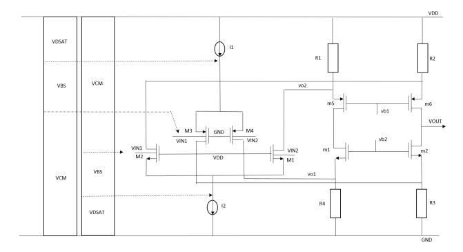
Figure 3.6 Folded cascoded OTA with bulk-driven rail-to-rail input
