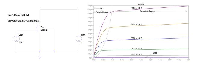
Figure 2.2: a) Biasing of 180nm NMOS b) Simulation for DC characteristics in LTSpice
