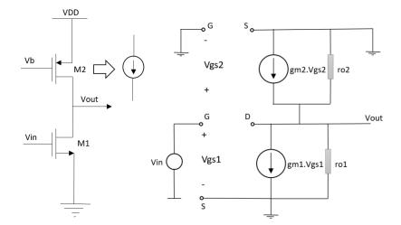
Figure 2.6: a) Circuit for CS stage with current source load b) AC analysis [36]
