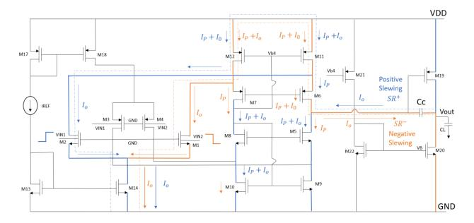
Figure 4.9: Simplified circuit during the positive and negative slewing
