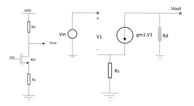
Figure 2.10: a) CS stage with source degeneration b) AC analysis [36]
