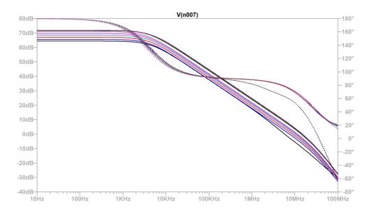
Figure 5.7: Bode plot for gain and phase of first stage
