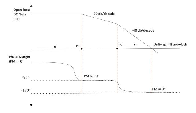
*Figure 4.5: Problems for gain and phase without compensation capacitor*
