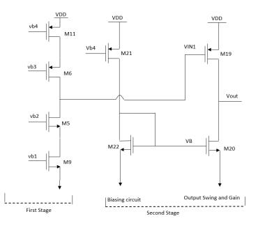
Figure 3.9 Biasing circuit for the second stage OTA
