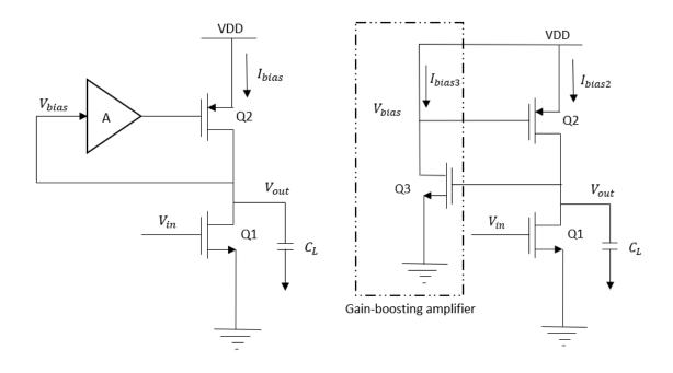
Figure 1.1: Gain boosting amplifier [14]
