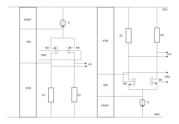
Figure 3.4 Input common mode range for PMOS and NMOS bulk-driven input stage
