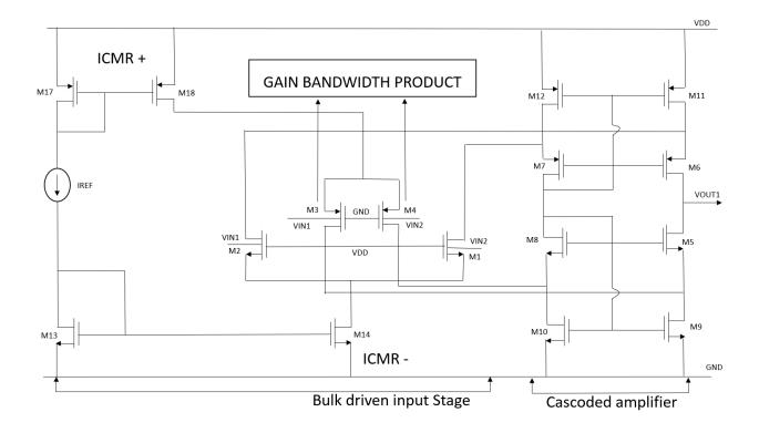
Figure 4.2: Circuit diagram of the first stage of OTA
