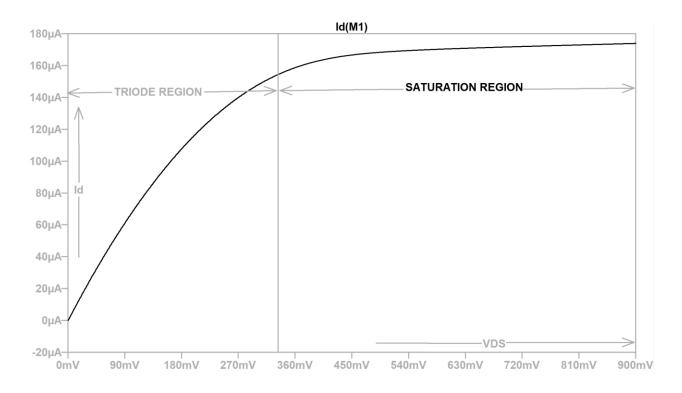
Figure 5.3: IV characteristics of the NMOS (variation of VDS from 0 to 0.9V at VBS = 0.4V)
