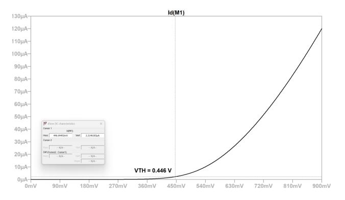
Threshold voltage,  $V_{th} = 446 \ mV$ .
