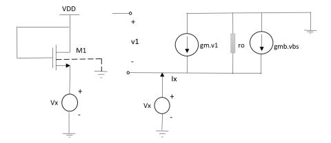
Figure 2.5: a) CS stage with diode connected load circuit b) AC circuit [36]
