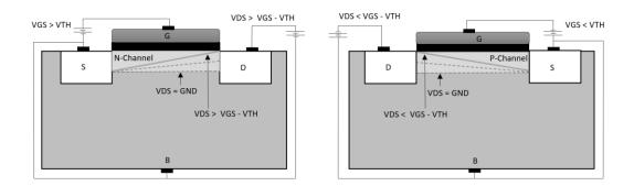
Figure 2.1: Cross-section of a) NMOS b) PMOS [36]
