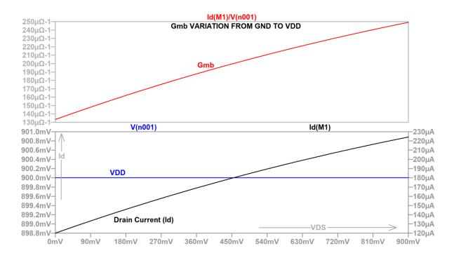
Figure 5.5: Variation of bulk driven NMOS intrinsic transconductance over the input common
