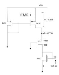
Figure 4.10: Equivalent circuit for ICMR<sup>+</sup> calculation
