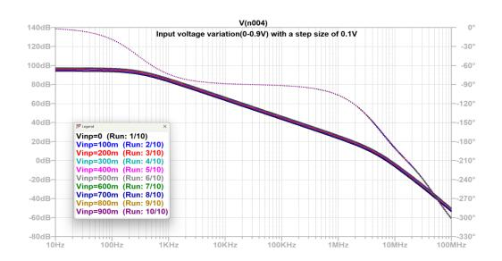
The effects of input voltage on the device performance while keeping the supply voltage is studied next.
