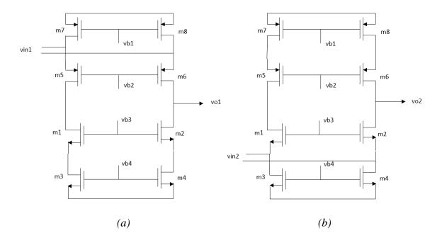
Figure 3.5 Folded cascoded OTA with a) NMOS input b) PMOS input
