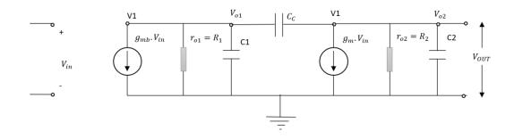
Figure 4.7: Small-signal analysis of the 2-stage OTA with the miller capacitance
