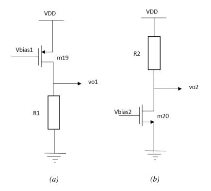
Figure 3.7 Common-source amplifier using a) PMOS b) NMOS
