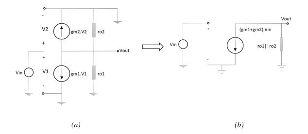
*Figure 2.8: a) Small-signal analysis for complementary CS stage b) Equivalent circuit [36]*
