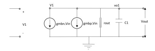
Figure 4.3: Small-signal analysis of the first stage
