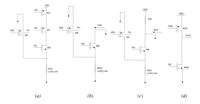
Figure 4.8 a) Half equivalent circuit for gain stage b)  $G_m$  calculation c)  $R_{out}$  calculation d) Equivalent circuit for calculation for gain in second stage
