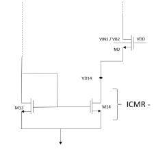
Figure 4.11: Equivalent circuit for ICMR<sup>-</sup> calculation
