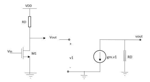
Figure 2.3: a) Common-source (CS) amplifier with resistive load b) AC analysis [36]
