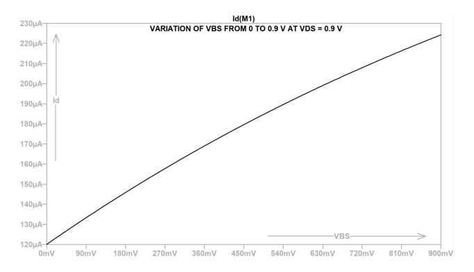
Figure 5.4: DC sweep for bulk driven NMOS (variation of VBS from 0 to 0.9V at VDS = 0.9V)
