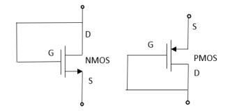
Figure 2.4: Diode connected a) NMOS b) PMOS
