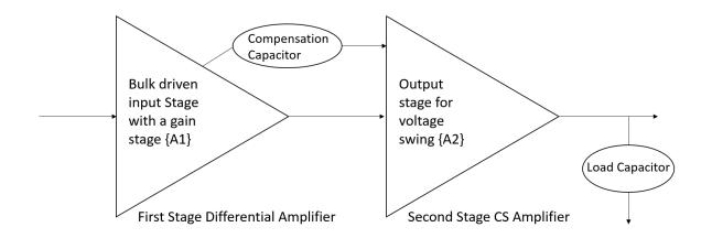
Figure 4.1: Block diagram of the 2-stage OTA
