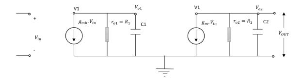
Figure 4.4: Small-signal analysis of the 2-stage OTA without the miller capacitance
