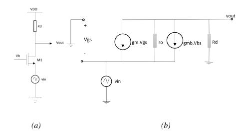
Figure 2.13: a) Common-gate circuit b) AC analysis [36]
