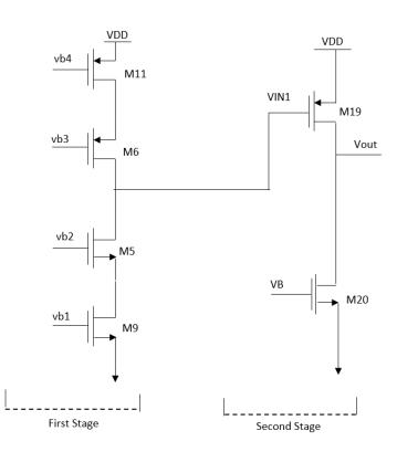
Figure 3.8 Second stage for the OTA using a PMOS common source configuration with current
