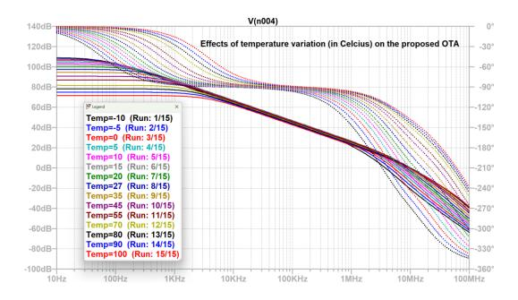
Figure 5.14: Effect of variation in temperature on gain and phase
