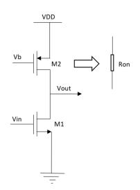
Figure 2.9: CS stage with triode load
