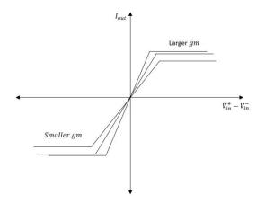
Figure 3.1 I/O characteristics of generic OTA [22]
