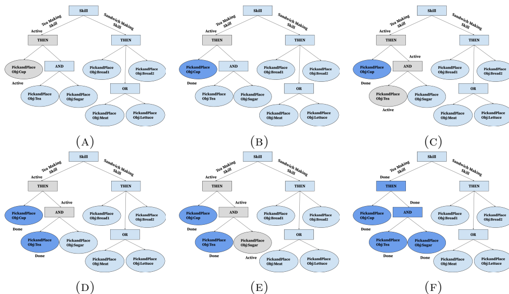
FIGURE 7.6: Order of execution for Tea Making Skill - (( Place Cup ) THEN (( Place Tea ) AND ( Place Sugar ))). After the SKILL node chooses the Tea Making Skill to execute, it only proceeds to execute the nodes that fall under the Tea Making Skill. (a) The THEN node for the Tea Making Skill under the SKILL component is invoked, which initiates the PickAndPlace node for the Cup object, (b) the state of the PickAndPlace of the Cup is changed to Done when the robot finishes placing the cup, (c) AND node gets activated and proceeds to activate the PickAndPlace node for the Tea which makes the robot starts pouring Tea into the cup, (d) the state of the PickAndPlace action of the Tea is changed to Done when the robot finishes pouring Tea and places it on the table, (e) PickAndPlace node for the Sugar under the AND node is activated which makes the robot adding sugar into the cup, (f) PickAndPlace action for the Sugar is Done when the robot places the Sugar on the table, and by doing this the state of all the active nodes under the Tea Making Skill is changed to Done.
