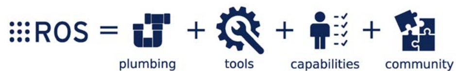
Figure 1. The ROS ecosystem is composed of multiple elements: (i) plumbing: a message-passing system for communication; (ii) tools: a set of development tools to accelerate and support application development; (iii) capabilities: drivers, algorithms, user interfaces as building blocks for applications; (iv) community: a large, diverse, and global community of students, hobbyists and multinational corporations and government agencies.
