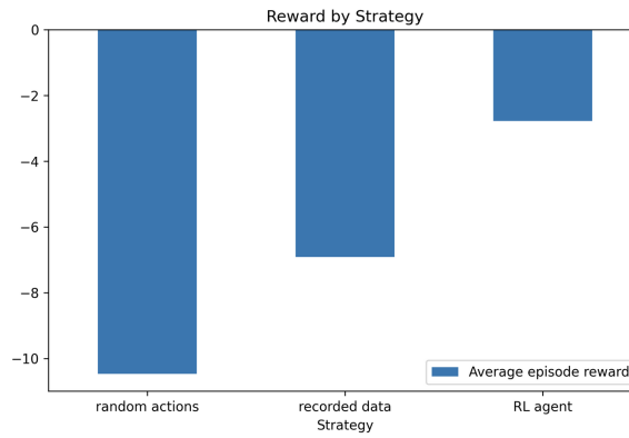
Figure 6: Comparison of rewards achieved by different strategies (higher is better). The given values are the mean episode rewards achieved in a test environment over 1000 episodes, where one episode covers a full plant growth cycle from 3% to 95% of maximal plant area.
