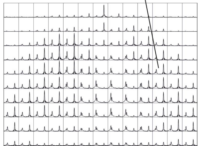
FIGURE 3 Example ^{129}\text{Xe} 3D MRSI results in the lung of 1 healthy volunteer at 1.5 T. Top: The data-analysis process for one of the unphased spectra via a triple Lorentzian fitting of the real and imaginary components. Bottom: A montage of the spectra in one coronal slice. The data were reconstructed to the original acquired resolution of 14 \times 14 \times 7 , and a zoom was applied in the frequency and spatial domains in this figure for clarity. In this slice, the trachea can be seen at the top, where a prominent gas peak is clearly visible in the corresponding spectra. For the pixels covering the heart, the RBC peak represents the main component
