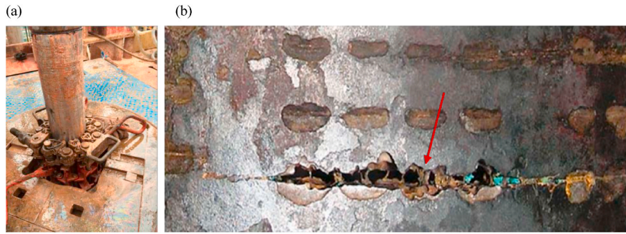
Fig. 1. (a) A schematic view showing the DP-slip system, where the slip is installed in the rotary table and used to suspend the DP; (b) Example of DP failure due to action of the slip inserts, where permanent die marks are shown on the external surface of the DP body and corrosion perforation (shown by the arrow) appears due to the die marks. Adopted from Albdiry and Almensory (2016) .
