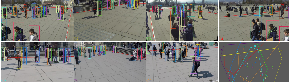
Fig. 5. The detection results at frame 1960 of the EPFL WILDTRACK dataset: (top row) from left to right, camera views C1, C2, C3 and C4; (bottom row) camera views C5, C6, C7 and the top view.
