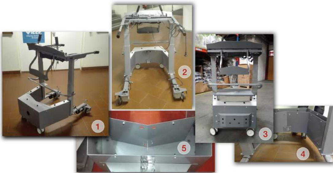
Figure 107: Walker's mechanical frame: (1)(2)(3) Walker's frame in different perspectives; (4) Interior section of the frame; (5) Walker's compartment that will contain all the electric system.
