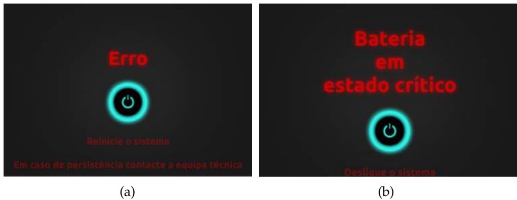
Figure 145: Local GUI shutdown warnings: (a) Communication with the Low-Level Controller lost; (b) Battery's voltage in critical state.
