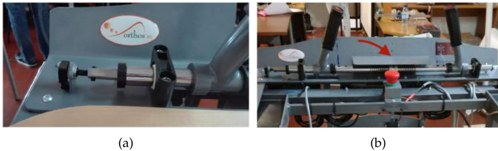
Figure 115: (a) Angular potentiometer coupled in the device; (b) Linear potentiometer below the mechanical piece pointed by the red arrow.
