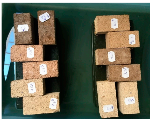
Figure 5. Specimens cut and accommodated over the saturated Oasis.
