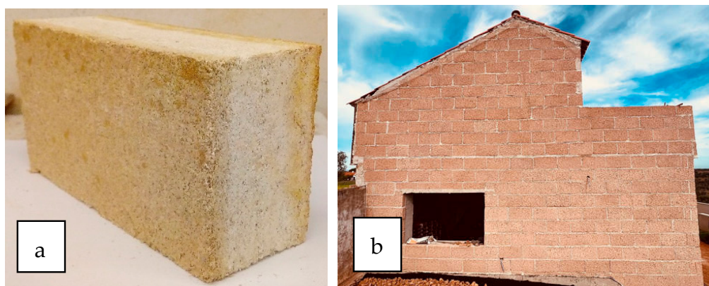
Figure 13. (a) Block with SCB and lime (credits: Souza [46]); (b) house with hemp concrete blocks (credits: Cãnhamor [47]).
