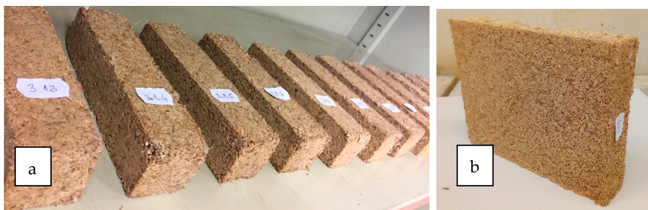
Figure 4. (a,b). Specimens for general tests (a) and sample for thermal conductivity (b).
