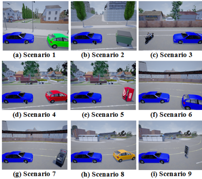
Fig. 4: Simulated stationary-obstacle scenarios used in the collision-avoidance experiments: (a) location A, green car; (b) location B, garbage container; (c) location B, motorcycle; (d) location C, red car; (e) location C, vending machine; (f) location D, blue car; (g) location D, ATM machine; (h) location E, orange car; (i) location E, street-sign.
