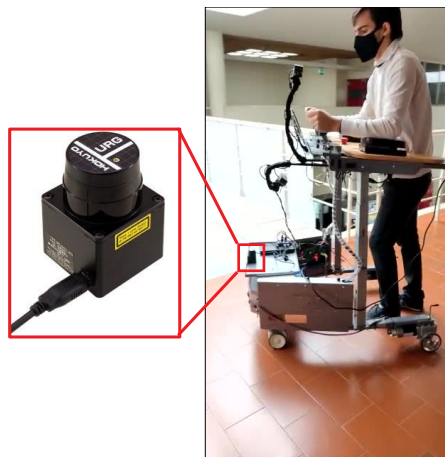
Figure 6.2: Photo of the Hokuyo's scanning rangefinder URG-04LX-UG01 and its positioning in the walker.
