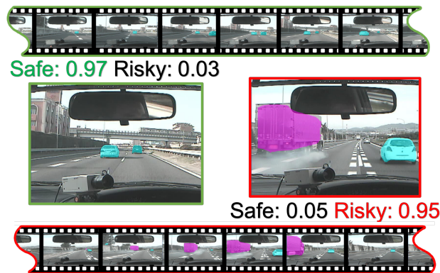
Figure 2.4: Two lane change samples and classification outputs of the system proposed by Yurtsever et al. [3].
