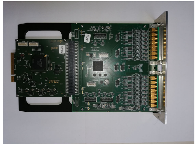
Fig. 7 New multi-channel electronic card FQT-TAMEX3. The card consists of two boards which are plugged together via a multi-pin connector. The board on the right is the front-end-electronics FQT and on the left one can see the FPGA-TDC TameX
