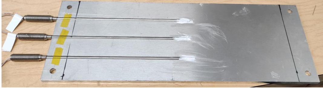
Fig. 54. Fixing of the thermocouples on the aluminium plates. Black lines identify the area that will be covered by the graphite sheets.
