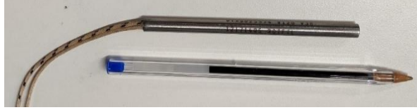
Fig. 65. Rotfil heating cartridge 36 V, 120 W, 6.5x100 mm. Pen for scale.
