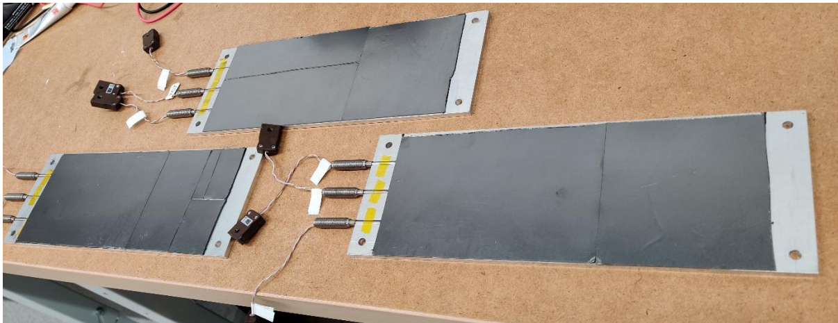
Fig. 55. Assembly of thermocouples and graphite completed for the three cell halves.
