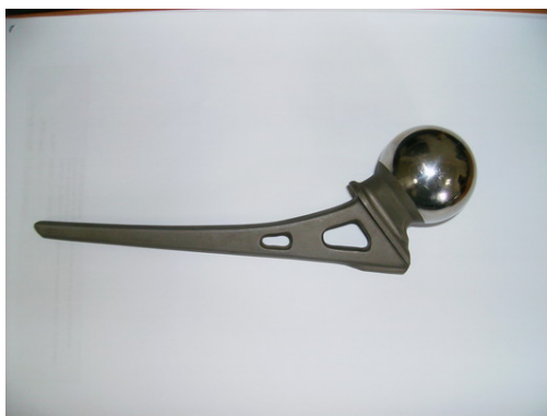
Fig. 1. Artificial hip joint prepared only by mechanical polishing of the surface.
