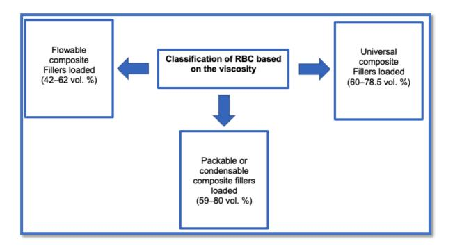
Figure 2-14: Classification of resin-based composite based on viscosity
