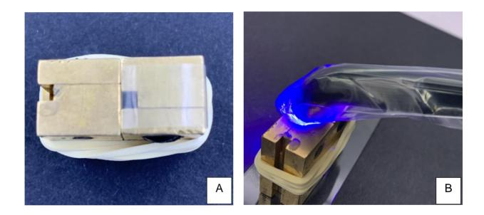
A. Top view of the mould with the Mylar strip and slot pressed using the back of another mould, and held with a rubber band
