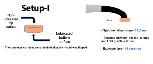
Setup one simulates the lubricated bottom surface of the upper increment
