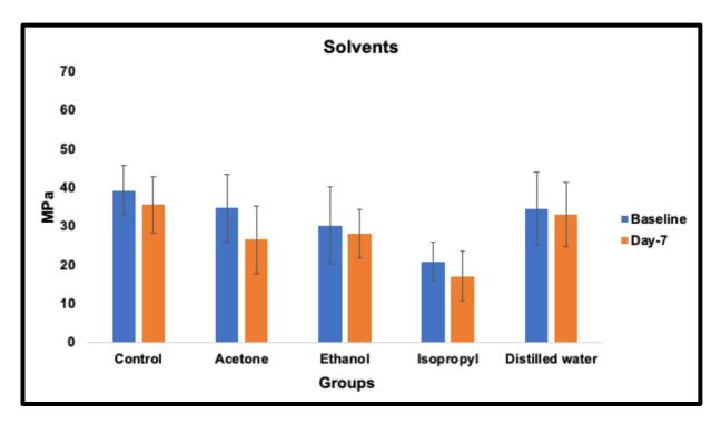
**Figure 6-9:** Mean and standard deviation values for the microtensile strength of Filtek RBC treated with solvents as ILs
