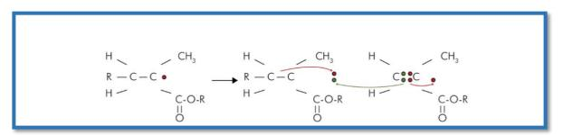
Figure 2-4: Polymer chain propagation from Rueggeberg et al., 2017
