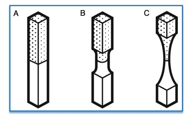
**Figure 2-21:** Different shapes of the micro-tensile test specimens: (A) Untrimmed; (B) Trimmed stick-shaped; (C) dumbbell and hourglass taken from Armstrong *et al.*, 2017
