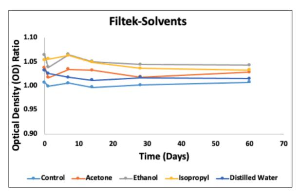
Figure 5-24: Optical density ratio of solvents over time for Filtek
