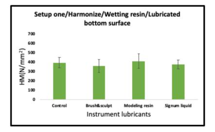
Figure 5-40: Mean and standard deviation values for tests of Martens hardness (Filtek & Harmonize) for non-lubricated top surface and wetting resin-lubricated bottom surface in setup one
