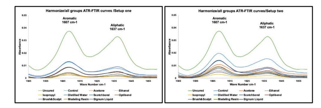
**Figure 5-31:** The FTIR scans for uncured and cured specimens of all tested Harmonize RBC groups for setup one and two. Also, the aromatic and aliphatic peaks that were used to calculate the DC.
