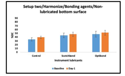
Figure 5-36: Mean and standard deviation values for the degree of conversion for Filtek and Harmonize for bonding agents-lubricated top surface and non-lubricated bottom surface/setup two
