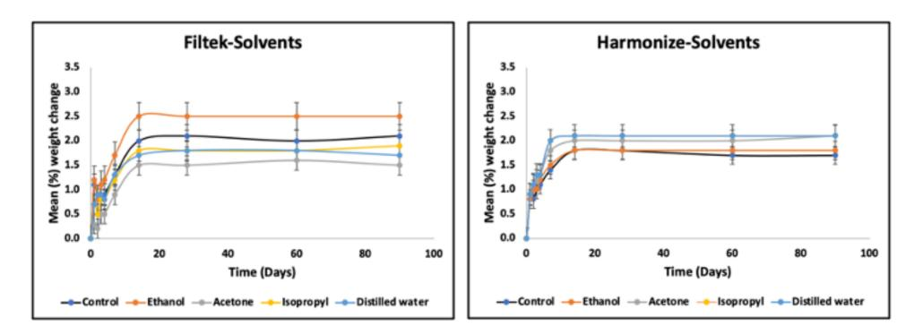
Figure 5-44: Solvent group % means for weight change and standard deviation for water uptake for Filtek and Harmonize stored in distilled water <90 days
