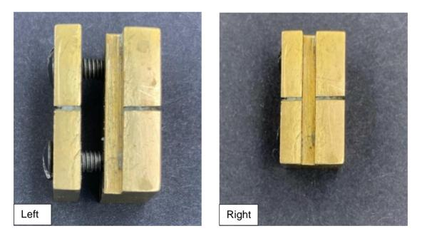
Figure 5-2: Left: Separated mould parts; Right: Assembled mould and a view of the mould slot
