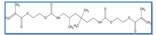
Figure 2-7: Chemical structure of UDMA from Floyd and Dickens, 2006
