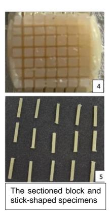
**Figure 6-4:** (1) The built-up RBC block; (2) Block attached to the saw arm to begin sectioning; (3) The low speed saw used to section the RBC block; (4) & (5) the sectioned block and stick-shaped specimens
