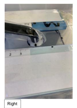
**Figure 5-16:** Right: The base fabricated to standardise the curing of the resin-based composite and the reference points on the mould, base and LCU tip to standerdise the position of the mould and LCU tip throughout all specimens; Left: The wheel used to adjust the height of the LCU tip in relation to specimen top surface
