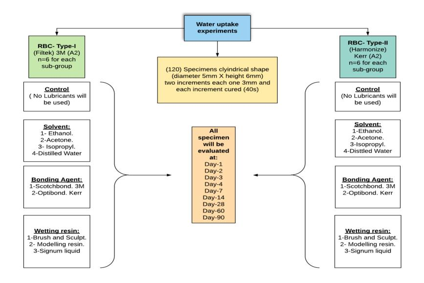
Figure 5-7: Specimen dimensions and key data for the water uptake experiments
