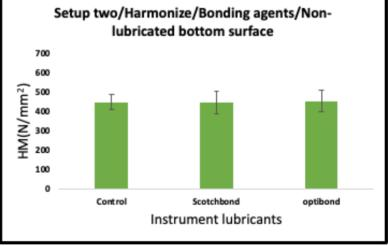
Figure 5-42: Mean and standard deviation values for Martens hardness tests (Filtek & Harmonize) for bonding agent-lubricated top surface and non-lubricated bottom surface in setup two
