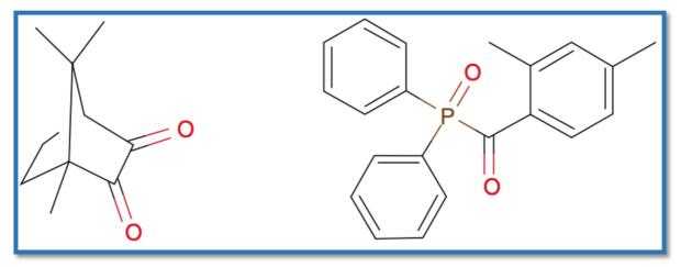
**Figure 2-102-11:** (A) The chemical structures of CQ and (B) TPO alternative photoinitiators of RBCs from Miletic, 2017
