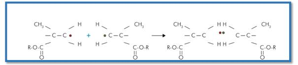
Figure 2-5: Chain termination due to free radical collision from Rueggeberg et al., 2017
