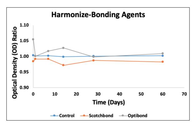
Figure 5-27: Optical density ratio of bonding agents over time for Harmonize
