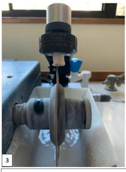
The low-speed saw used to section the RBC block
