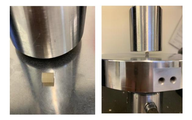
Figure 5-20: Position of the DTS specimens under compression
