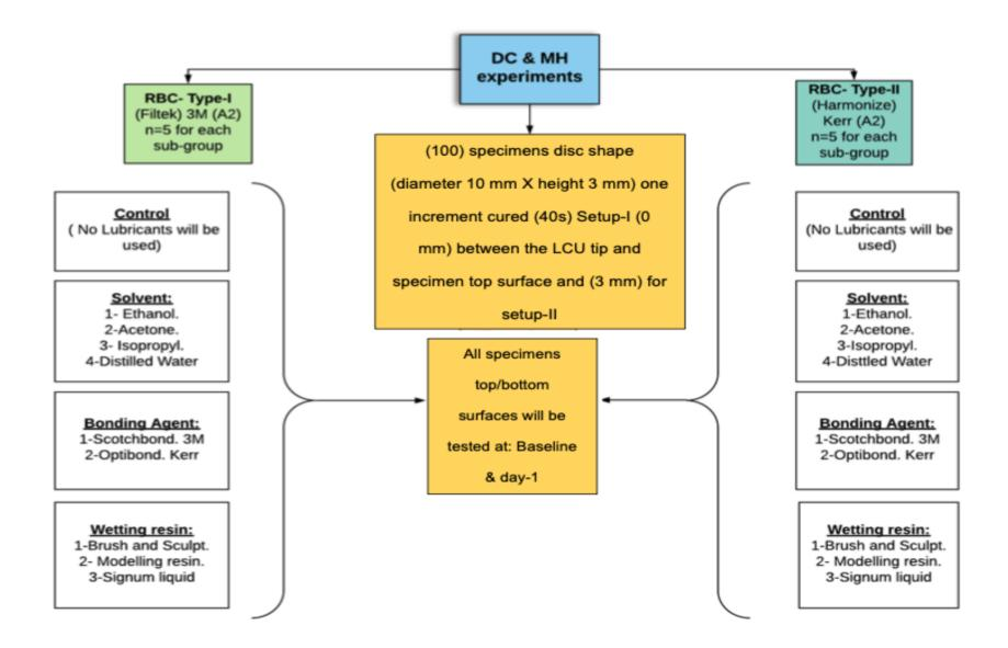
Figure 5-9: Specimen dimensions and key data for the degree of conversion and hardness experiments
