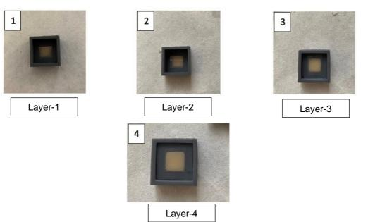
**Figure 6-3:** Steps in building up the block using the multiple layer mould; four layers (1-4) were filled with RBC and each cured with the LED LCU
