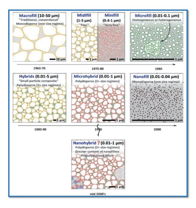
Figure 2-12: Classification of resin-based composite on the filler size taken from Miletic, 2017
