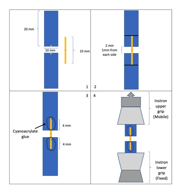
Figure 6-7: The reference points and the position of the tested specimens, and the area glued with cyanoacrylate glue
