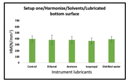
Figure 5-38: Mean and standard deviation values for Martens hardness tests (Filtek & Harmonize) on non-lubricated top surface and solvent-lubricated bottom surface in setup one
