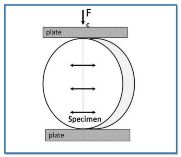
Figure 2-20: The diametral tensile test from Ilie et al., 2017
