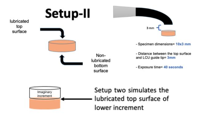
**Figure 5-15:** Setup two, showing the degree of conversion and Martens hardness tests on the specimen top lubricated surface and bottom non-lubricated surface
