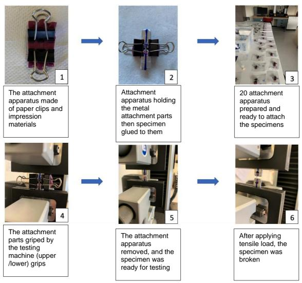
Figure 6-8: The attachment pieces and specimen testing steps
