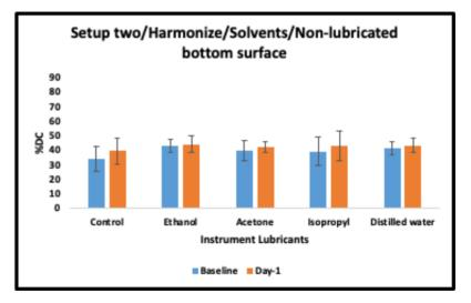
Figure 5-35: Mean and standard deviation values for the degree of conversion for Filtek and Harmonize for solvents-lubricated top surface and non-lubricated bottom surface/setup two
