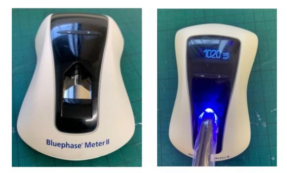
Figure 5-1: Bluephase Meter II and irradiance measuring of the LED LCU
