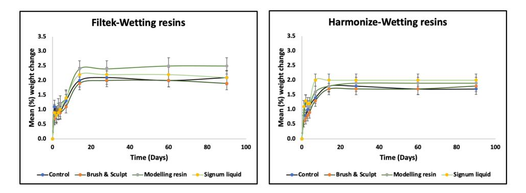
Figure 5-46: Wetting resin group mean % weight change and standard deviation of water uptake for Filtek and Harmonize, stored in distilled water <90 days
