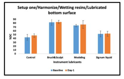
Figure 5-34: Mean and standard deviation values for the degree of conversion for Filtek and Harmonize for non-lubricated top surface and wetting resins-lubricated bottom surface/setup one
