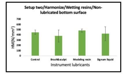
Figure 5-43: Mean and standard deviation values for Martens hardness tests (Filtek & Harmonize) for wetting resin-lubricated top surface and non-lubricated bottom surface in setup two
