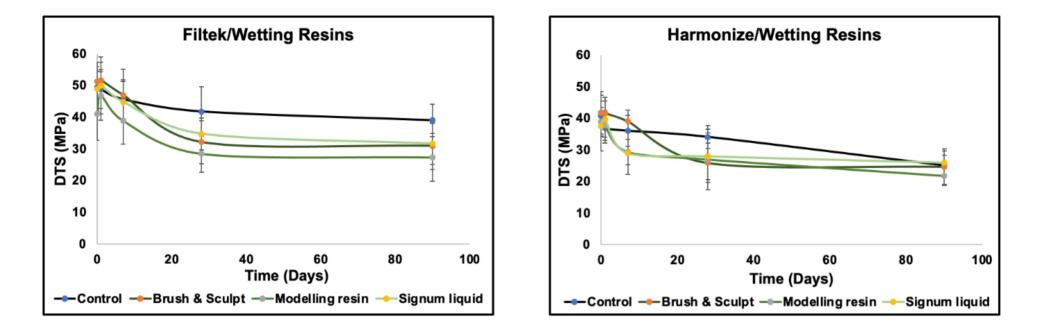
**Figure 5-49:** Wetting resin group mean (MPa) DTS and standard deviation values for Filtek and Harmonize, stored in distilled water <90 days
