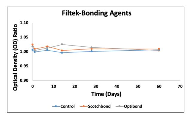
Figure 5-26: Optical density ratio of the bonding agents over time for Filtek
