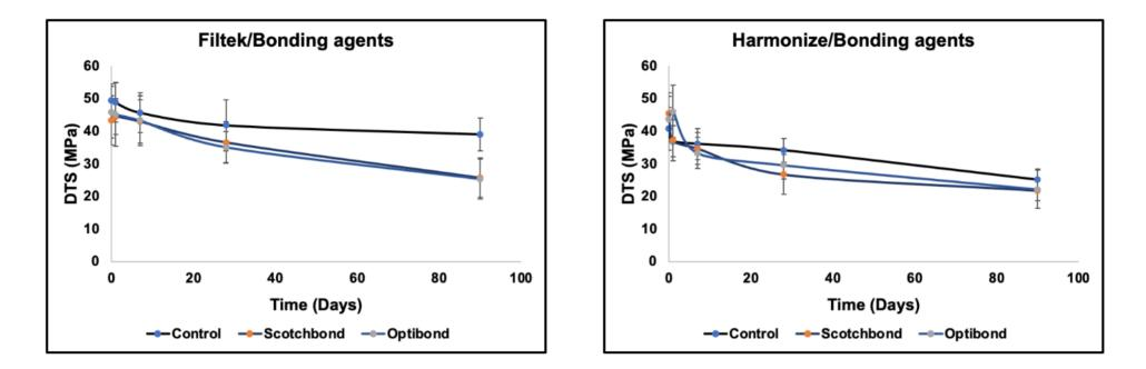
Figure 5-48: Bonding agent group mean (MPa) and standard deviation DTS for Filtek and Harmonize, stored in distilled water <90 days
