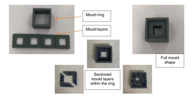
Figure 6-1: The final shape of the mould's layers and holding ring
