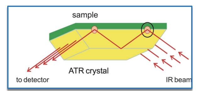
Figure 2-18: Attenuated total reflection in contact with a sample from Bruker, 2011
