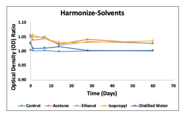
Figure 5-25: Optical density ratio of solvents over time for Harmonize
