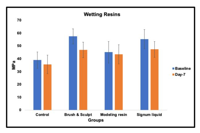
**Figure 6-11:** Mean and standard deviation values for the microtensile strength of Filtek RBC treated with wetting resins as ILs
