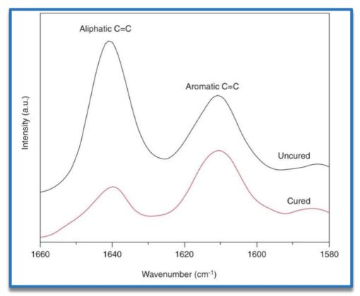
**Figure 2-19:** The reference bands aromatic 1,607 cm<sup>-1</sup> and aliphatic 1,637 cm<sup>-1</sup> of the infrared used to determine the DC of cured/uncured RBCs taken from Miletic, 2017
