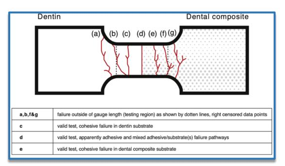
**Figure 2-22:** Fracture failures in specimens by location taken from (Armstrong *et al.*, 2017)
