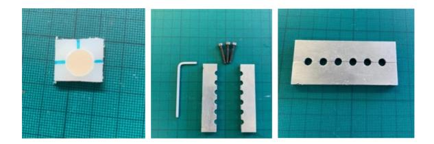
**Figure 5-11:** Left: polytetrafluoroethylene (PTFE) mould for the DC and HM specimen preparation; Centre and Right: stainless steel attachable mould for COIIA, DTS and WU specimens' preparation
