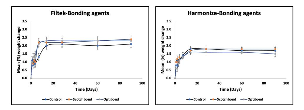
Figure 5-45: Bonding agent group means of % weight change and standard deviation for the water uptake in Filtek and Harmonize, stored in distilled water <90 days
