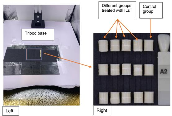
**Figure 5-18:** Left: Interior of the professional photo light box and tripod; Right: Arrangement of the groups of specimens in the photo light box
