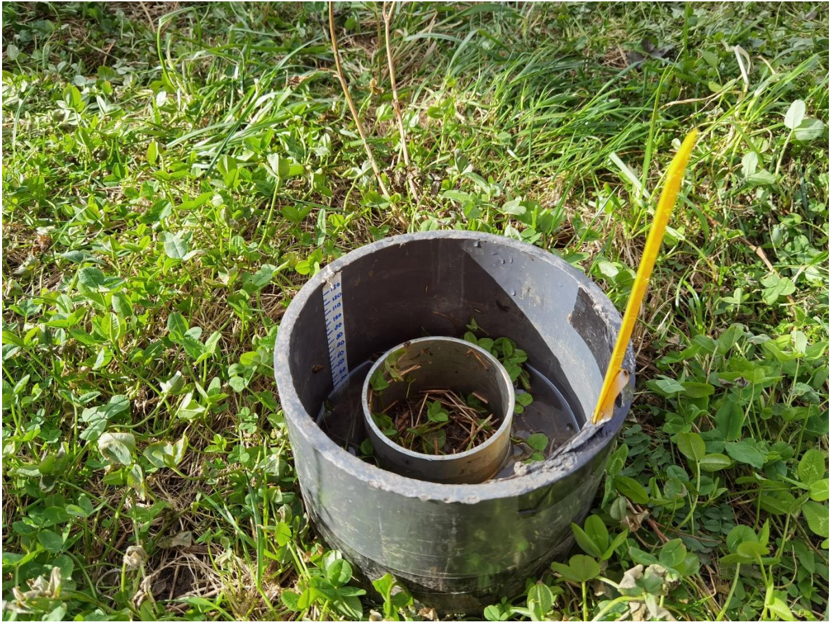
Figure C. 1 Image of a double ring infiltrometer used in the lysimeters. (Image Jiaqian Wang)
