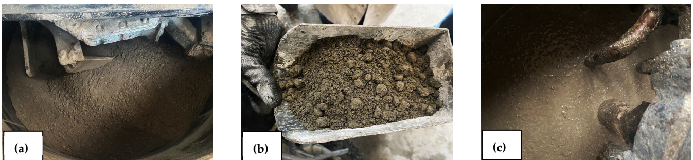
Figure 2. Mix procedure: dry mix of the aggregates (a); addition of first part of mixing water (b); settling of the SCC mix by 3 min (c).
