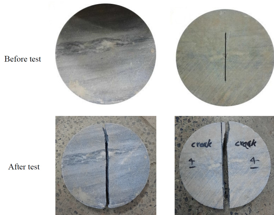
Figure 4. BD (left) and CBD (right) samples tested to determine the tensile strength and the fracture toughness, before and after being tested.
