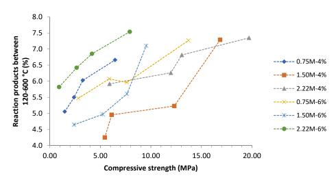
**Figure 13.** Relationship between reaction product percentages and compressive strength for each paste. For each curve (formulation), each point is the value for each curing time (1, 3, 7 and 28 days).
