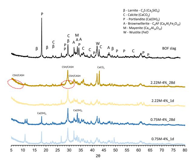
**Figure 10.** Comparison of the XRD patterns of 0.75M-4% (blue) and 2.22M-4% (yellow) at 1 and 28 days (dotted red circle: broad hump indicating amorphous phase structure).
