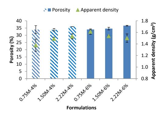
Figure 8. Apparent density and porosity of pastes.
