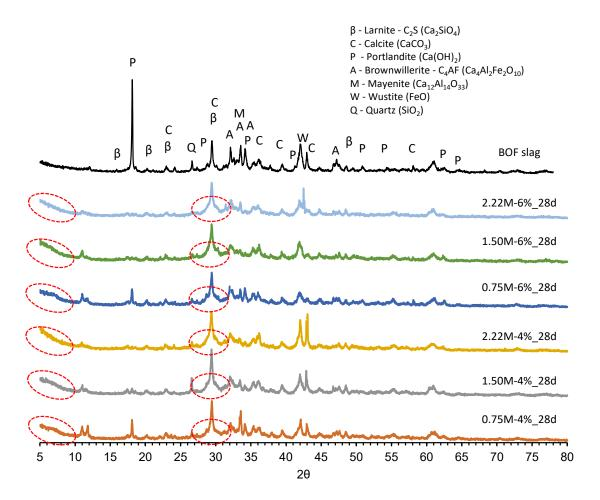
**Figure 9.** XRD patterns of pastes at 28 days (dotted red circle: broad hump indicating amorphous phase structure).
