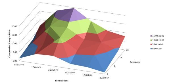
Figure 6. Compressive strength distribution with respect to the formulation and curing age.
