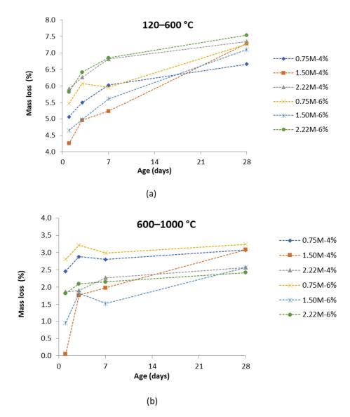
**Figure 12.** Mass losses (%) for all pastes after 1, 3, 7 and 28 days of curing in different temperature ranges: (a) 120–600 °C and (b) 600–1000 °C.
