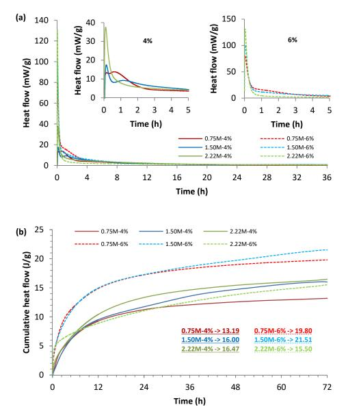
the silica modulus and  $Na_2O$  concentration in the activator clearly modified the BOF slag activation kinetics.
