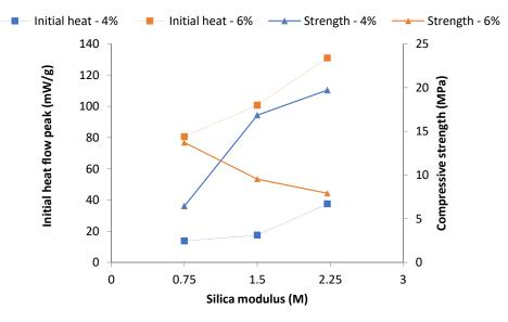
**Figure 7.** Influence of the activator parameters on the relation between the initial heat release and compressive strength (blue: 4% of Na<sub>2</sub>O; orange: 6% of Na<sub>2</sub>O; squares: initial heat release; triangles: compressive strength).
