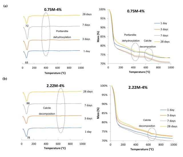
Figure 11. TG/DTG of (a) 0.75M-4% and (b) 2.22M-4%.
