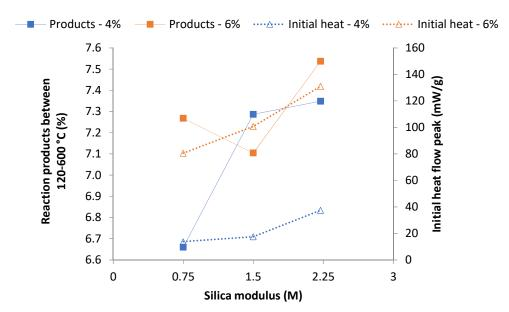
**Figure 14.** Influence of activator parameters on the relationship between the reaction products and the initial heat release (blue: 4% of Na<sub>2</sub>O; orange: 6% of Na<sub>2</sub>O; squares: reaction products; triangles: initial heat release).
