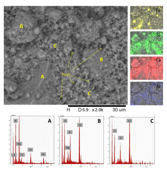
**Figure 15.** SEM image of 0.75M-4% (magnification of 2000×) with elemental mapping and EDX spectra of the scanning points: (**A**) RO phase, (**B**) calcium silicate (unreacted BOF slag particle) and (**C**) C-S-H (reaction product).
