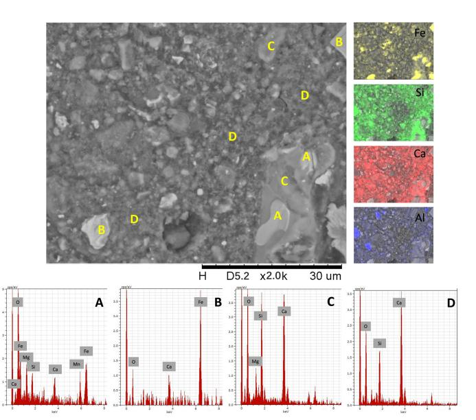
**Figure 16.** SEM image of 2.22M-4% (magnification of  $2000 \times$ ) with elemental mapping and EDX spectra of the scanning points: (**A**) RO phase (embedded in BOF particle), (**B**) steel particle, (**C**) calcium silicate (unreacted BOF slag particle) and (**D**) C-S-H (reaction product).
