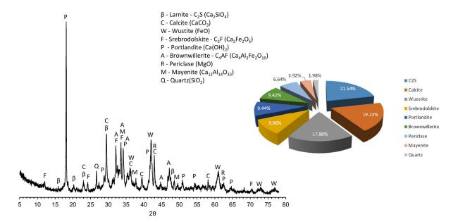
Figure 2. XRD pattern and Rietveld refinement.
