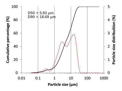
Figure 1. Particle size distribution of the BOF slag.
