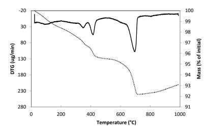
Figure 3. TG (dotted line) and DTG (solid line) diagrams of the BOF slag.
