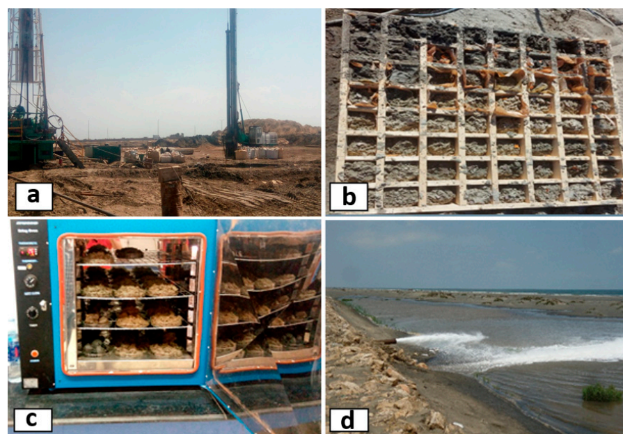
Figure 5. (a) Drilling of wells in the study area, (b) sediment samples during drilling of wells, (c) drying the sediment sample in the oven, and (d) during the pumping test of well.
