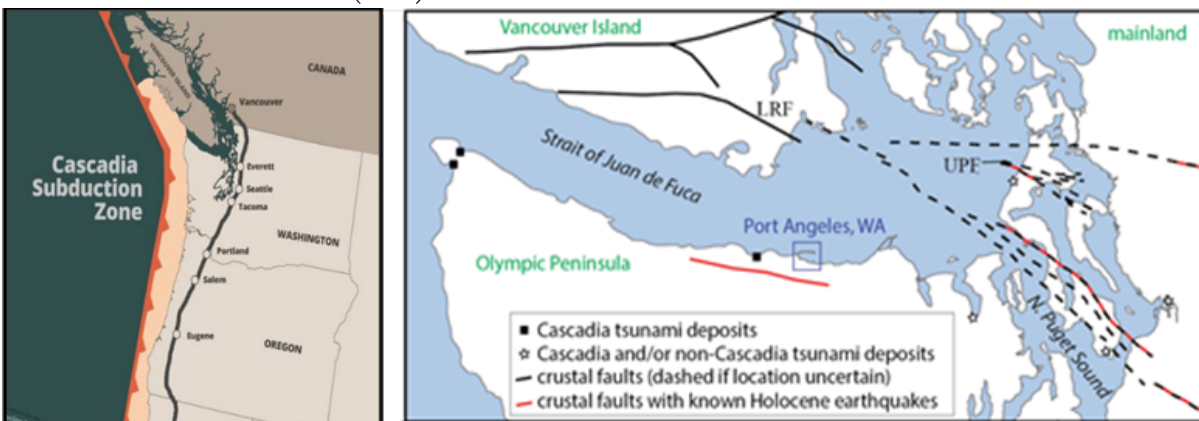
Figure 1. (LEFT). The CSZ (in orange) denotes where the Juan de Fuca plate is subducting below North America (from NOAA, 2019). (RIGHT). Part of Puget Sound, Washington with site area Port Angeles. Crustal fault traces marked by solid and dashed lines; LRF stands for Leech River fault and UPF stands for Utsalady Point fault. Sites with previously identified tsunami deposits near Port Angeles are shown by black squares or white stars (locations from Williams and Hutchinson, 2000; Williams et al., 2005; Hutchinson et al., 2013; Peterson et al., 2013).
