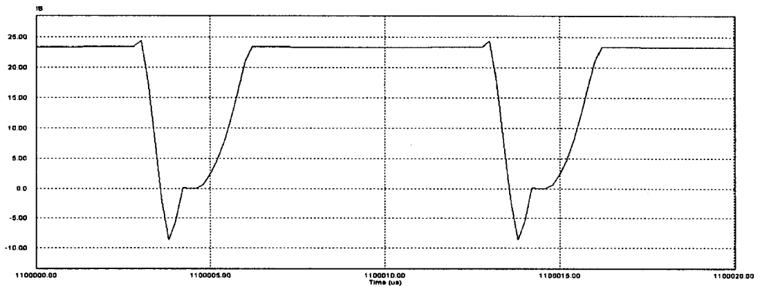
Fig.4.16 PSIM Simulation of the bridge input current I_{Lr1}
