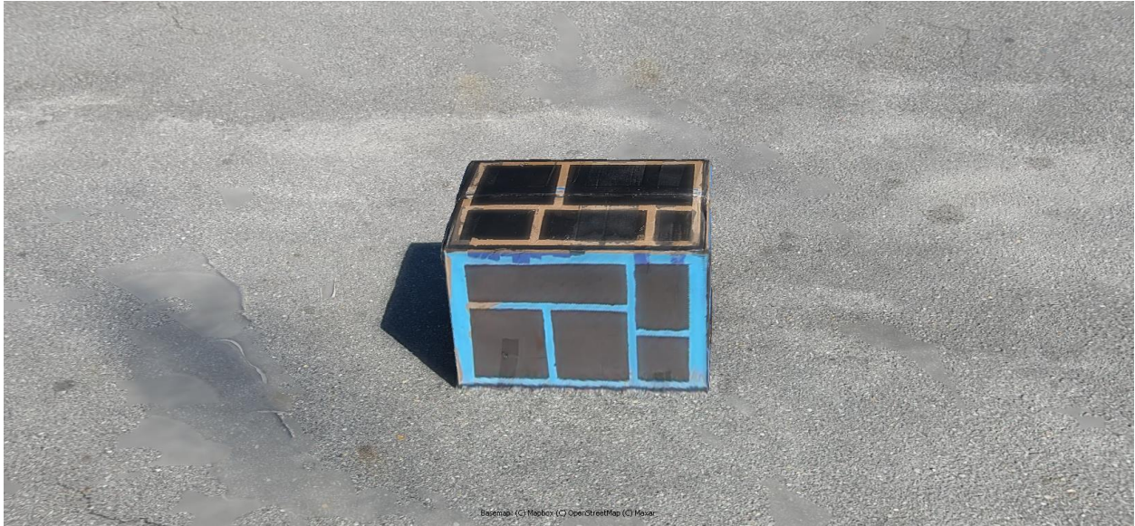
Figure 19: Initial test subject for system operation tests: a cardboard box with a painted grid.
