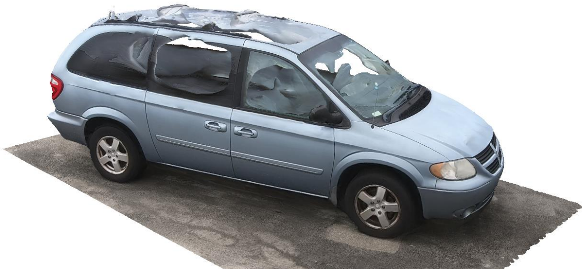
Figure 20: Model recreation errors displayed when using SFM on transparent material.
