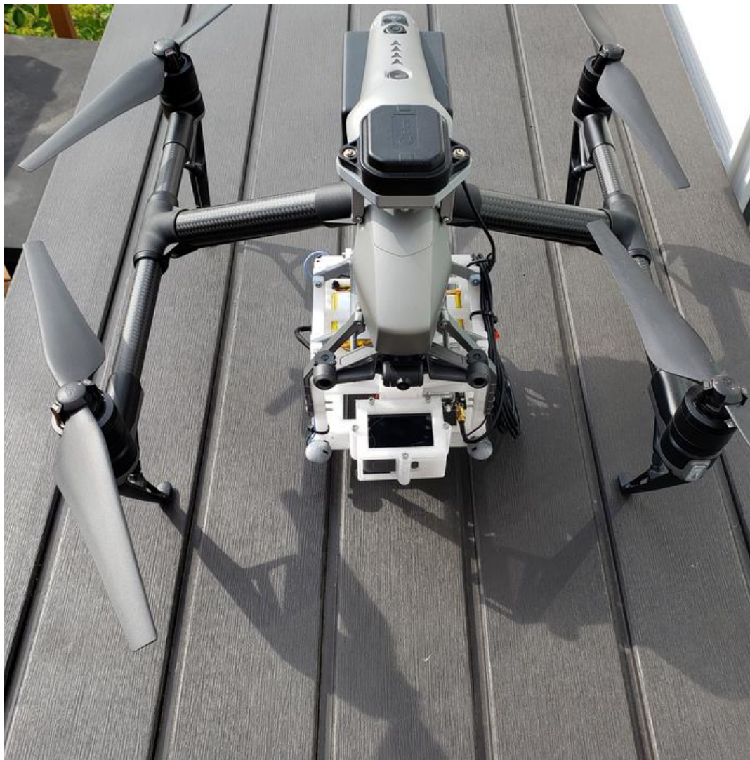
Figure 22: Final design of rover module as attached to DJI Inspire 2 Pro UAV.
