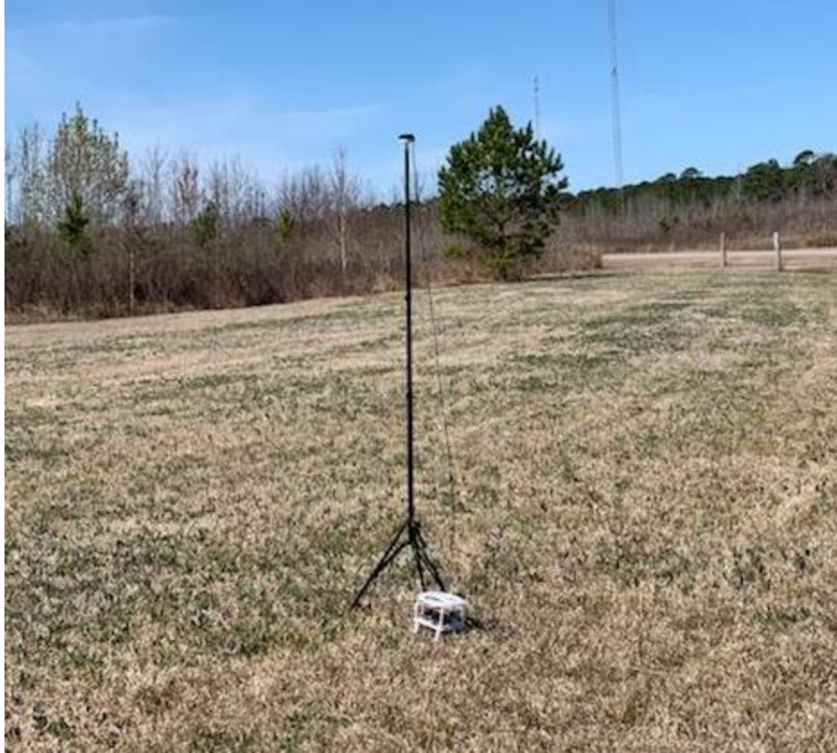
Figure 25: Base station GCP in use with antenna tripod during data collection.
