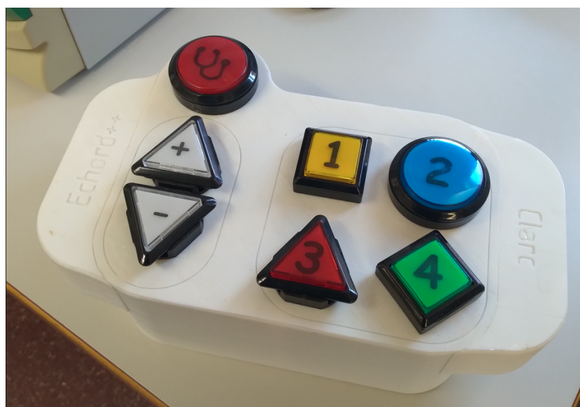
Figure 15. The final version of the remote control device. In both cases, the large buttons on the device are used by the user to express their choice of answer.
