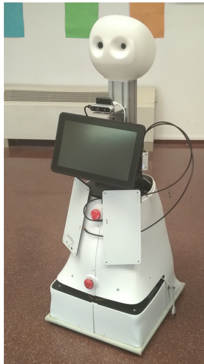
Figure 16. One of the CLARA robots with the two RFID antennas.
