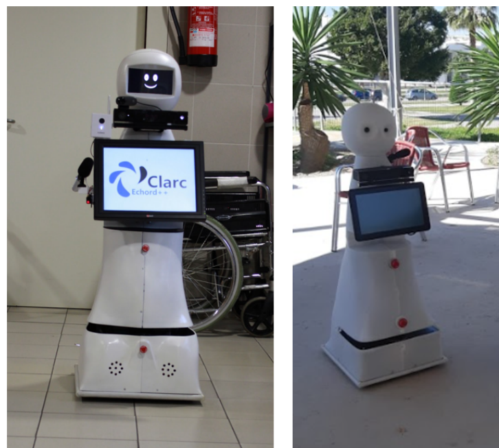
Figure 6. External aspect of CLARA after adding (left) a first version and (right) the second version of the external housing.
