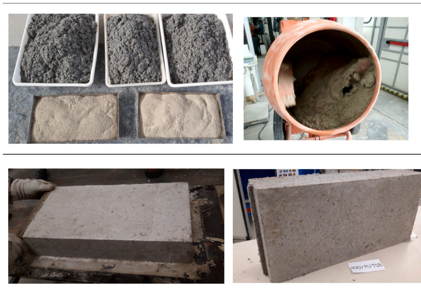
Fig. 2. Mortar blocks fabrication process. The eco-mortar blocks have dimensions of (50 x 25 x 10) cm 3 . In the case of tongue and groove joints, each piece has a slot (the groove) cut all along one edge with 1 cm deep and 2.5 cm wide, and a thin, deep ridge (the tongue) on the opposite edge with 1 cm deep and 2 cm wide.
