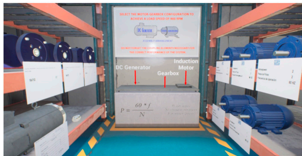
Figure 4. Induction motor arrangement design level.
