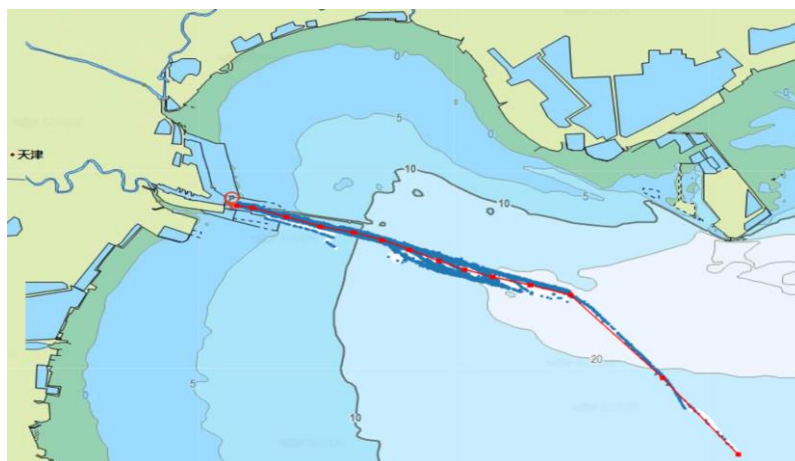
Fig. 19. Based on the massive AIS trajectory big data, inbound and outbound port routes optimization (Taking massive AIS trajectory big data of Tianjin Port of China as an example).
