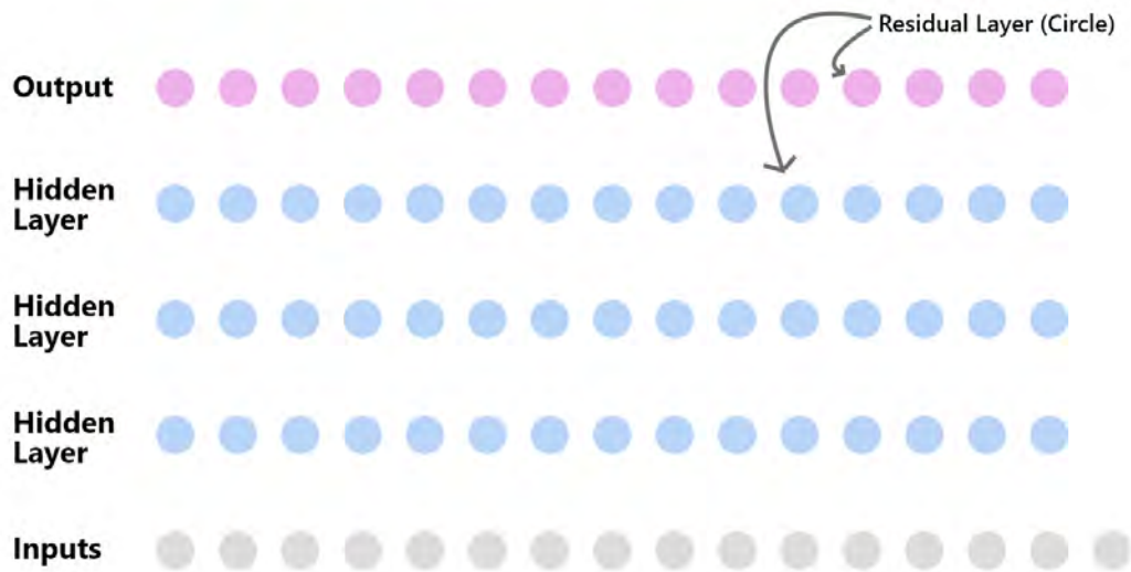
Fig. 4.8: Causal Convolution stack
