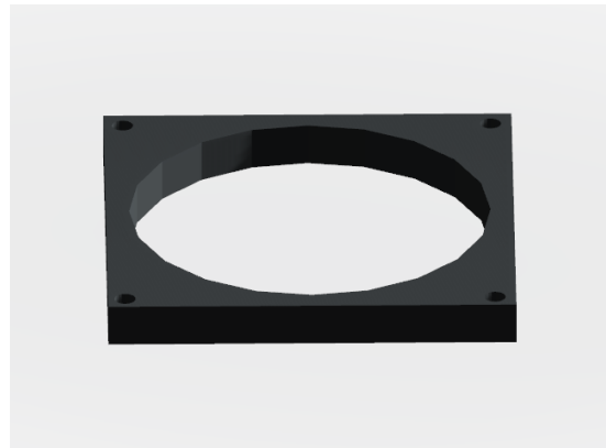
(b) CAD drawing of the acrylic part.
