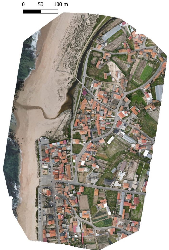
Figure 21 – Orthophotomap generated with WebODM, 4 GCPs.
