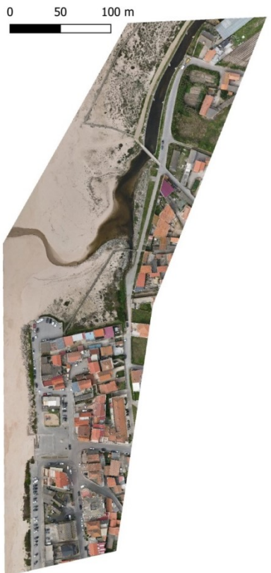
Figure 19 – Own survey (WebODM), pixel size: 0,038x0,038m
