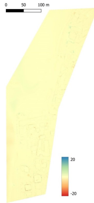
Figure 43 – Difference of DSMs (2022–2021), pixel size: 0,083x0,083m
