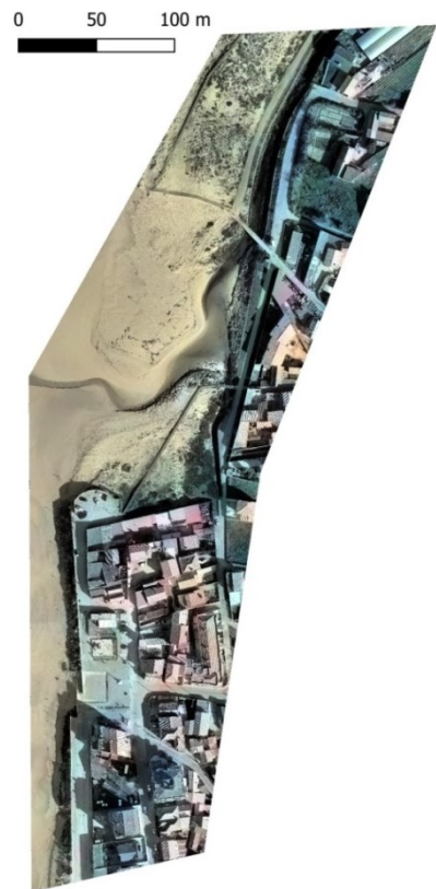
Figure 24 – Fused dataset, with RGB mask, pixel size: 0,025x0,025m
