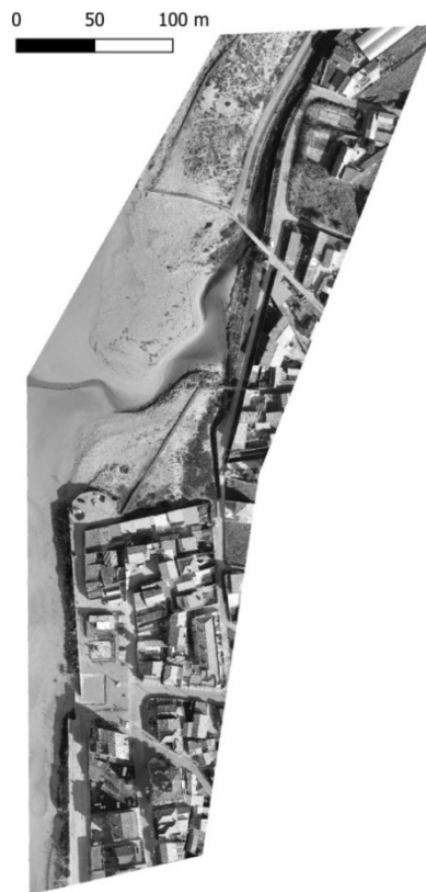
Figure 23 – Intensity “image”, obtained from APA's orthophotomap HSI transform, pixel size: 0,025x0,025m
