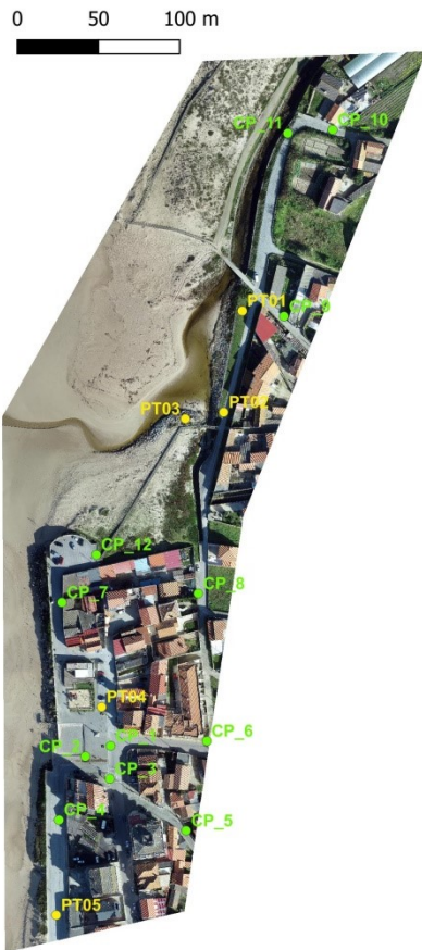
Figure 34 – Base map with 5 GCPs (yellow) and 12 Check Points (green)
