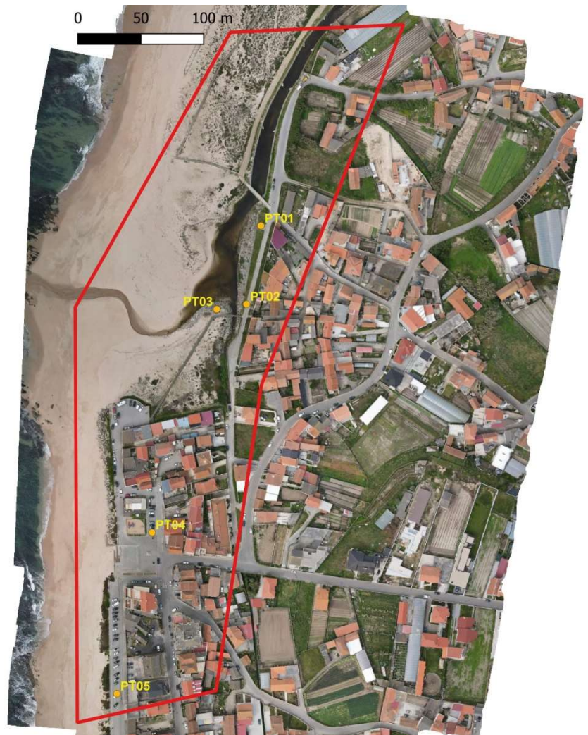
Figure 9 – Area of interest (own orthophotomap), with GCPs and clipping polygon overlaid.
