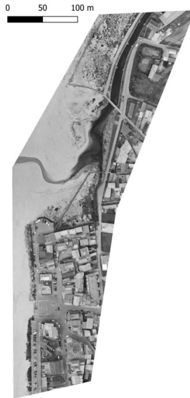
Figure 26 – Intensity "image", obtained from Agisoft's orthophotomap HSI transform, pixel size: 0,041x0,041m
