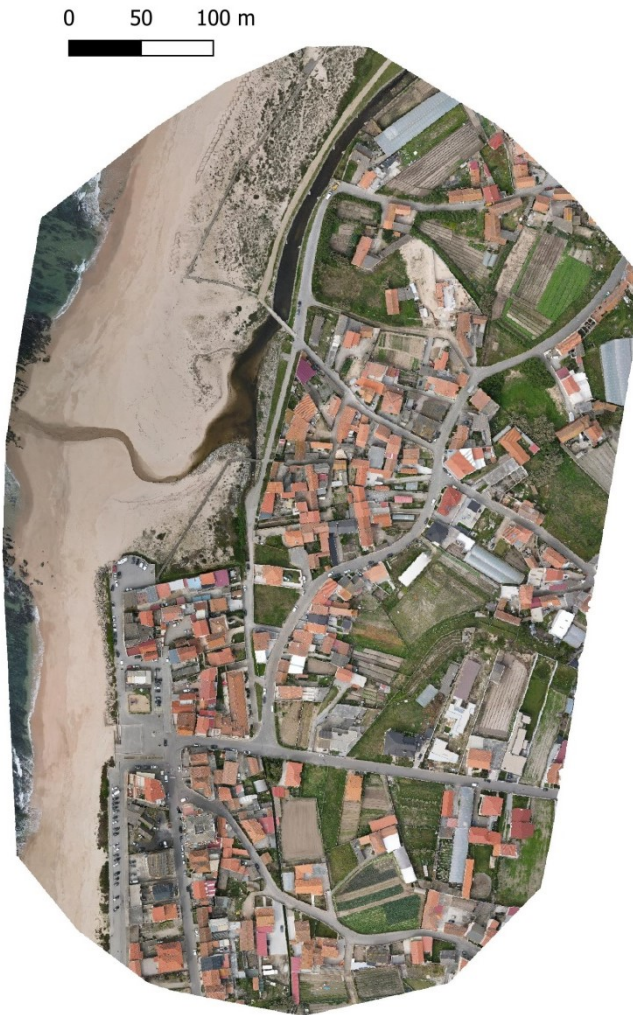
Figure 20 – Orthophotomap generated with WebODM, no GCPs.
