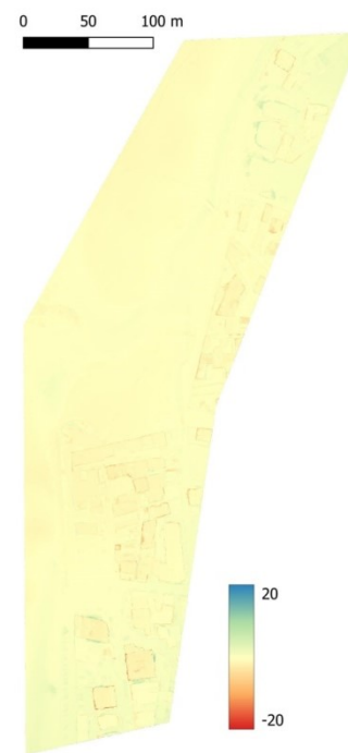
Figure 43 – Difference of DSMs (2022–2021), pixel size: 0,083x0,083m
