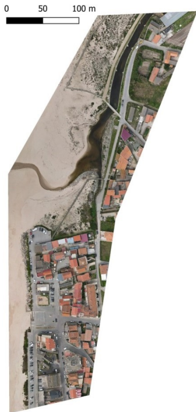
Figure 17 – Own survey (DSM – Agisoft ), pixel size: 0,042x0,042m
