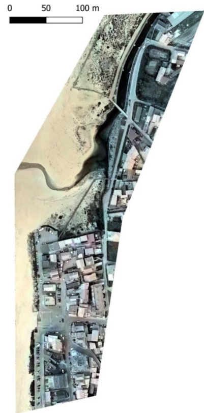
Figure 27 – Fused dataset (Satellite and Agisoft datasets) with RGB mask, pixel size: 0,041x0,041m
