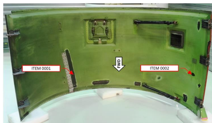
Figure 6. A320 fan cowl door damage identification spots. The repair procedures for these damages cannot be found in the aircraft maintenance manual.
