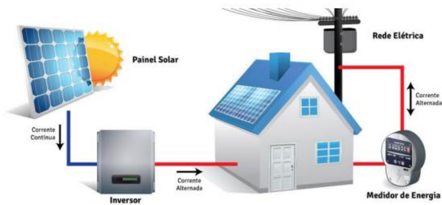
Figure 2 Grid-connected Photovoltaic System [8]
