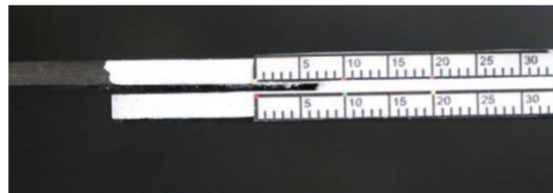
Figure 2. Painting of the specimen face and scale location to aid measuring the crack propagation.
