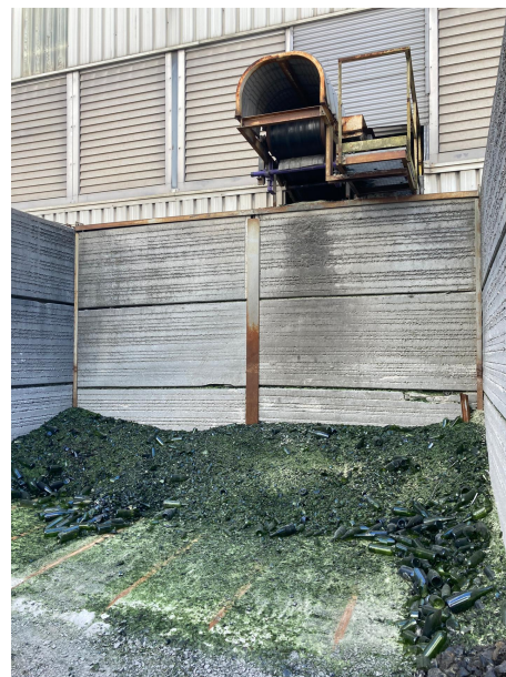
(b) Internal cullet from inspection machine rejections
