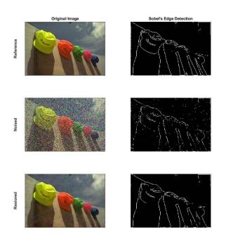
FIGURE 5: VISUAL COMPARISON OF EDGE DETECTION FOR ORIGINAL, NOISED, AND RESTORED EDGES FOR SOBEL EDGE DETECTION ALGORITHM [14]
