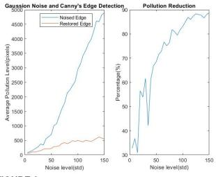
FIGURE 2: COMPARISON OF NOISE POLLUTION IN NOISED AND RESTORED EDGES FOR CANNY EDGE DETECTION ALGORITHM [14]
