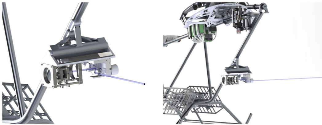
Figure 8. System mounted on the hoverbike. The transparent blue line represents the laser path.
